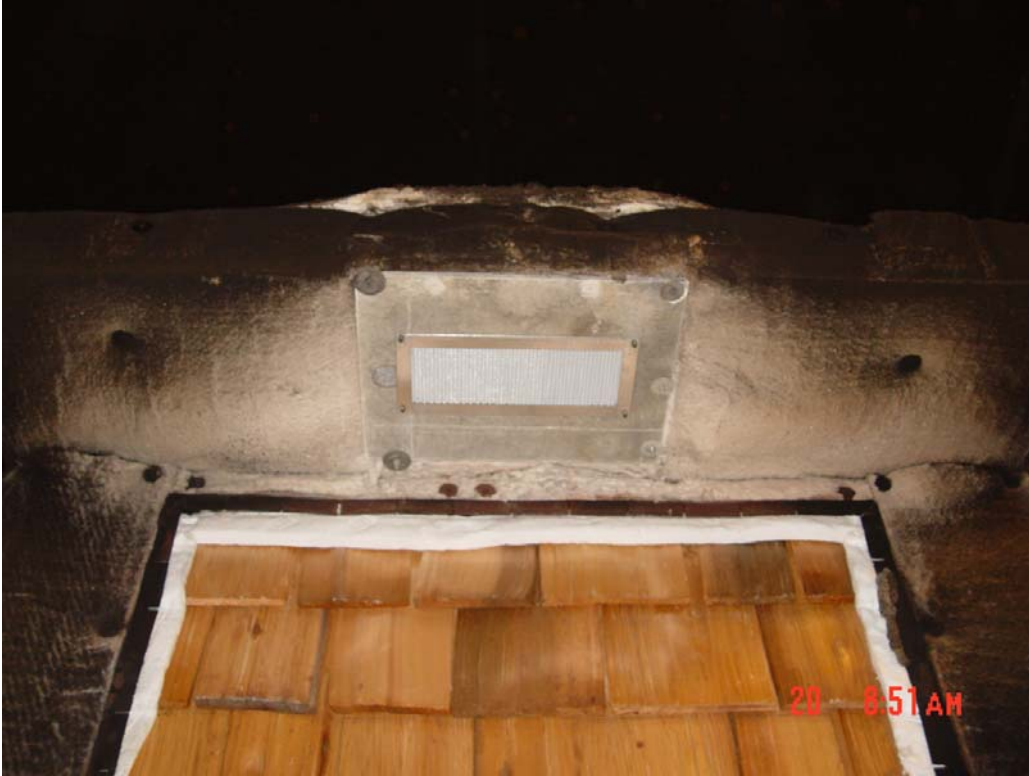
Vent in position prior to flame exposure
