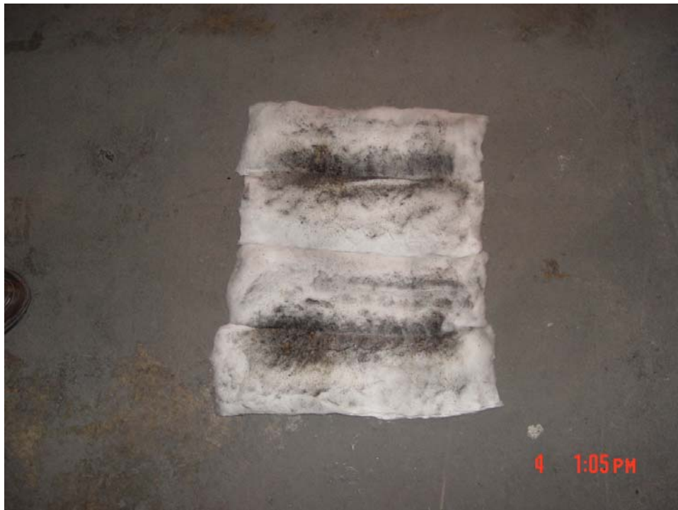
Two cotton targets showing ember distribution post test
